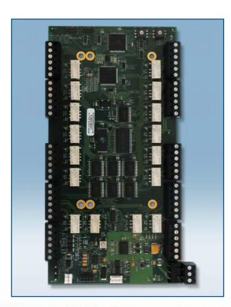
The ORC features 16 output relays and 1 tamper input. All applications are downloadable into FLASH memory thus eliminating the need to replace EPROMs for application changes and system upgrades.
