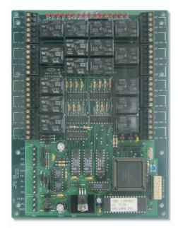
The Relay Output Controller (ROC) operating with a PointGuard X Security System Processor (SSP) provides command output capabilities to PointGuard X Software packages.
